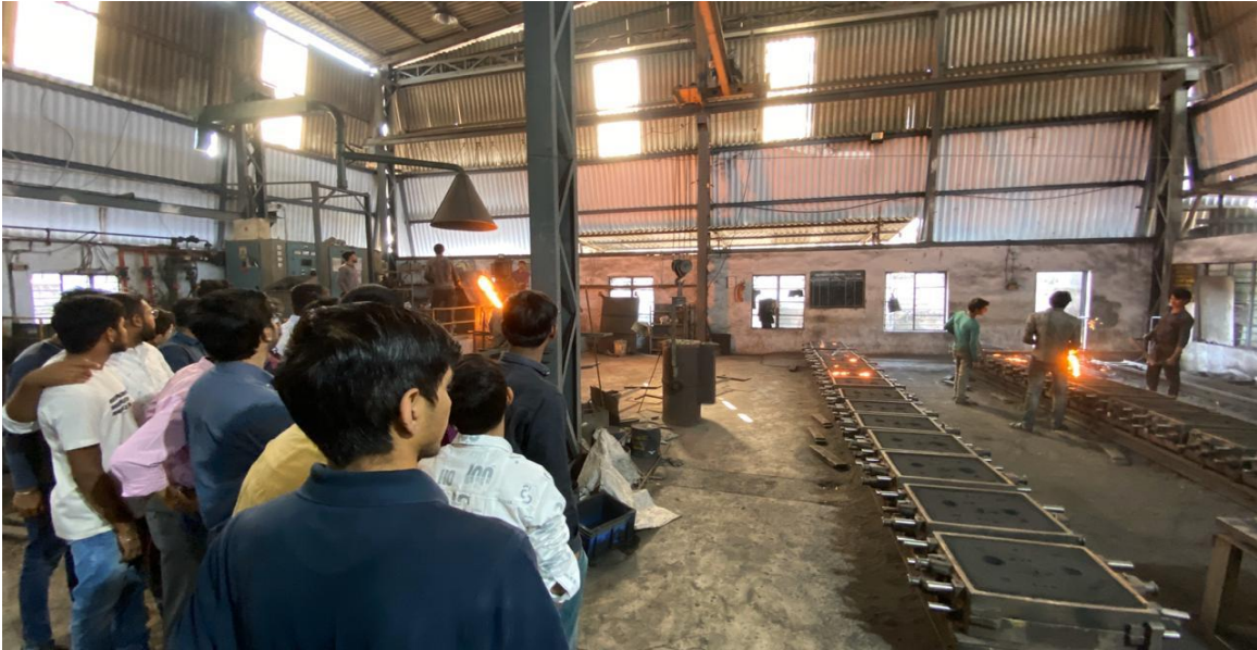
Fig: Pouring of molten metal in cavity
